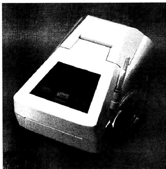
Fig. 1 : A thick film semiconductor (absorption effect transistor) gas monitor.
