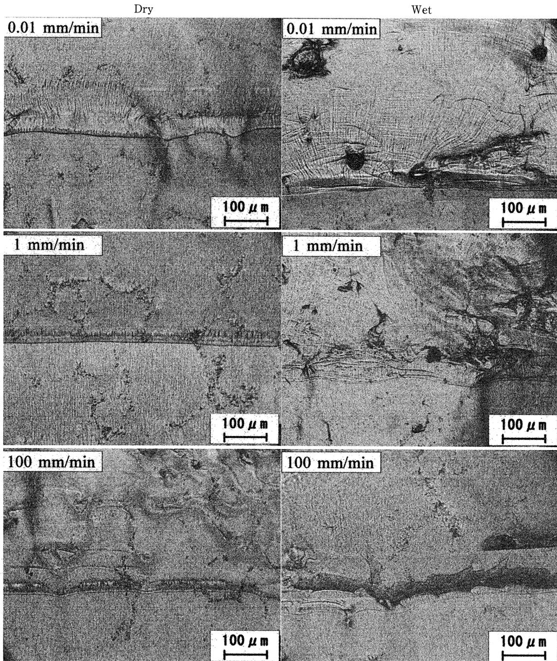
Fig. 5. Fracture surfaces after measurement of  $K_{IC}$
