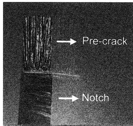
Fig. 2. Pre-crack initiated from the notch by the three point bend mode
