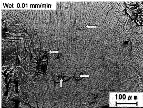
Fig. 6. Pattern created by SCG in wet specimen
