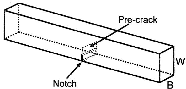
Fig. 1. Specimen configuration for the measurement of fracture toughness of heat cured denture base acrylic resin
