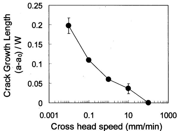
Fig. 3. Effect of cross head speeds on crack growth length in wet specimen
