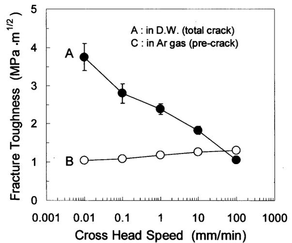
Fig. 4. Fracture toughness (K<sub>IC</sub>) of heat cured denture base acrylic resin A (wet specimen) and B (dry specimen) were measured in distilled water and Ar gas, and calculated using total crack length and pre-crack length, respectively.
