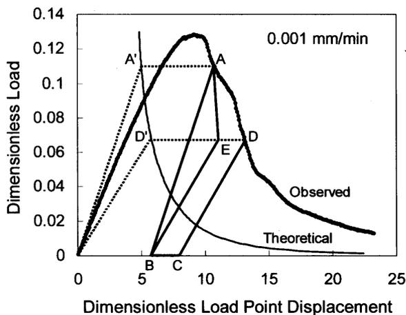
Fig. 5. Dimensionless load-loadpoint displacement curves of heat cured denture base resin (Observed) and the perfect elastic body (Theoretical).
