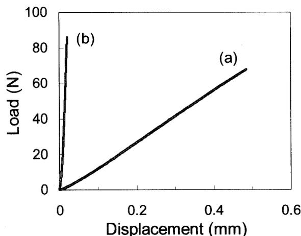
Fig. 2. Load-displacement curves at the cross head speed of 0.001 mm/min.
