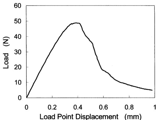
Fig. 3. Load-load point displacement curve in distilled water by the three point bend mode at the cross head speed of 0.001 mm/min.
