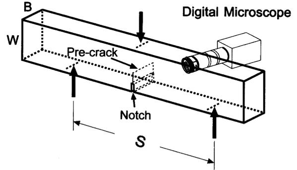
Fig. 1. Illustration of specimen for stable crack growth measurement.
