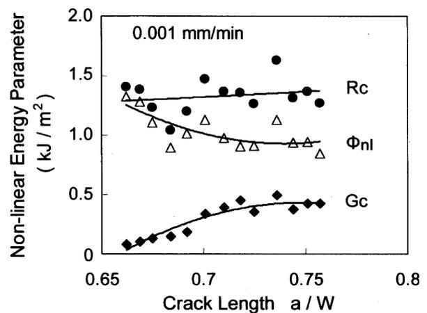
Fig. 6. Non-linear energy fracture parameters of heat cured denture base acrylic resin.
