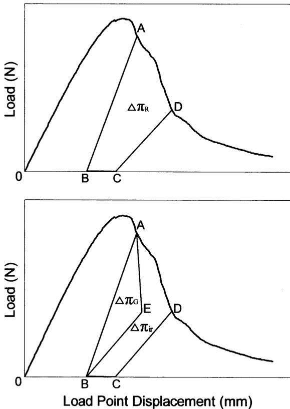
Fig. 4. Non-linear fracture parameters defined by unloading line AB and DC.
