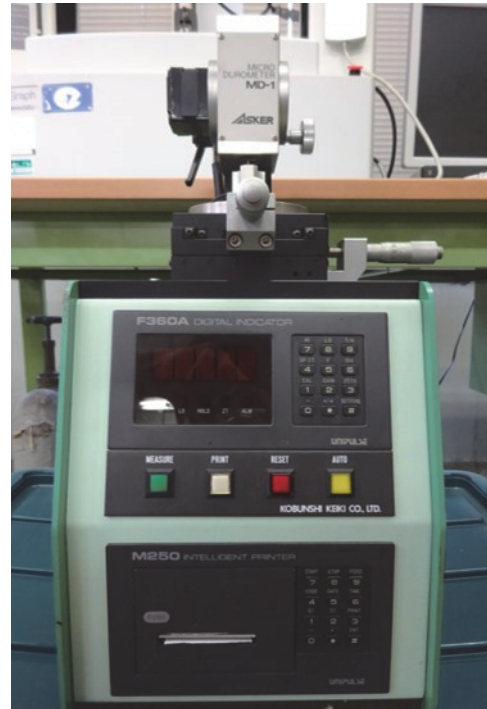
Fig. 2. Durometer (MD-1, Kobunshi Keiki Co Ltd, Kyoto, Japan)
