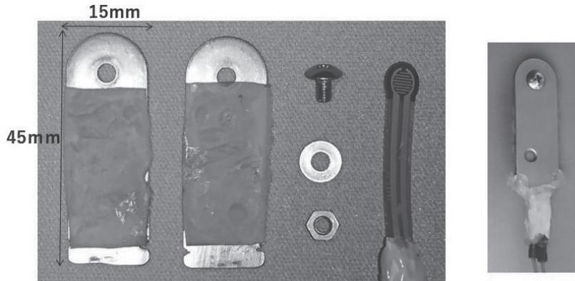
図2 The exploded view of the measuring terminal
