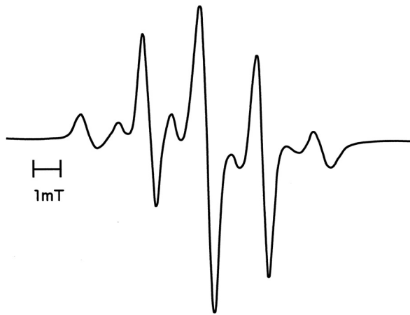
Fig. 3 Nine-line ESR spectrum of resin specimen after light irradiation
