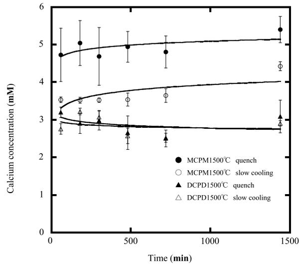
Fig. 5 Time dependence of concentration of Ca<sup>2+</sup> eluted from heated MCPM and DCPD in 200 mM acetic acid buffer solutions. For both MCPM and DCPD samples, two cooling conditions were employed, i.e., under one condition samples were slowly cooled down to the room temperature after heating at 1500 °C and under the other condition samples were quenched.
