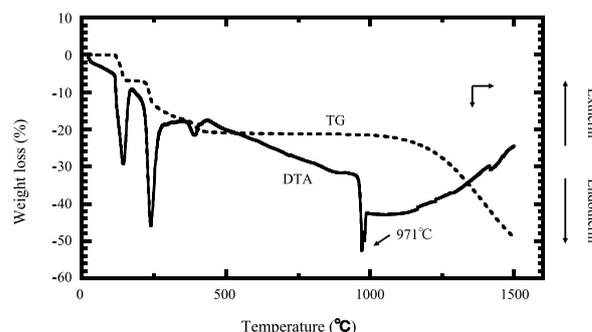
Fig. 1 Thermogravimetric and differential thermal analyses of MCPM
