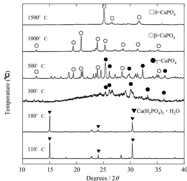
Fig. 3 X-ray diffraction patterns of MCPM heated at various temperatures
