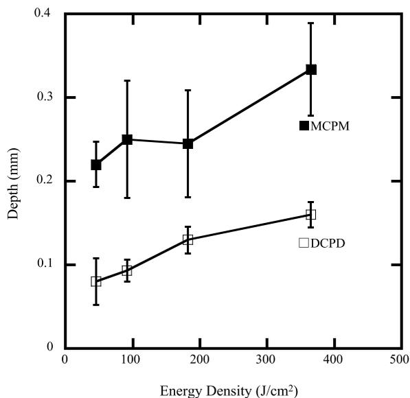
Fig. 10 Depth of laser spots of MCPM and DCPD disks at different energy densities.
