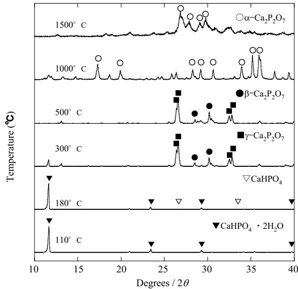
Fig. 4 X-ray diffraction patterns of DCPD heated at various temperatures
