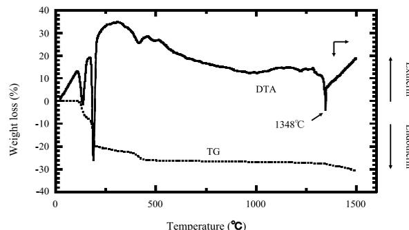
Fig. 2 Thermogravimetric and differential thermal analyses of DCPD
