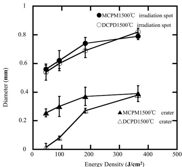
Fig. 9 Diameters of laser spots and craters of MCPM and DCPD disks at different energy densities
