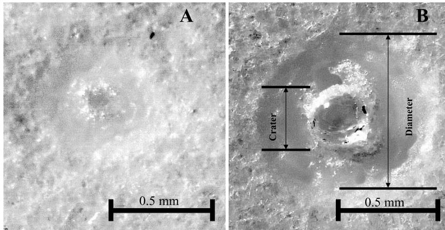
Fig. 6 Photo micrographs of lased spots formed on MCPM disks. Disks were laser-irradiated at an energy density of 45.6 J/cm<sup>2</sup> (1.0 W for 0.1 s) (A) and at an energy density of 365 J/cm<sup>2</sup> (8.0 W for 0.1 s) (B).
