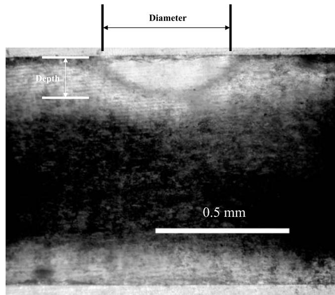
Fig. 8 A polarized light micrograph of a cross section of the spot of a DCPD disk that was CO<sub>2</sub>-lased at the energy density of  $91.2 \text{ J/cm}^2$  ( $1.0 \text{ W}$  for  $0.2 \text{ s}$ )
