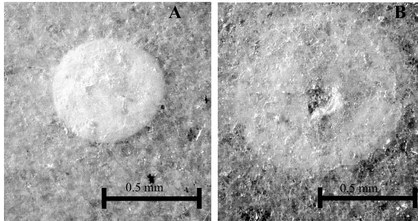
Fig. 7 Photo micrographs of lased spots formed on DCPD disks. Disks were laser-irradiated at an energy density of  $45.6 \text{ J/cm}^2$  ( $1.0 \text{ W}$  for  $0.1 \text{ s}$ ) (A) and at an energy density of  $365 \text{ J/cm}^2$  ( $8.0 \text{ W}$  for  $0.1 \text{ s}$ ) (B)
